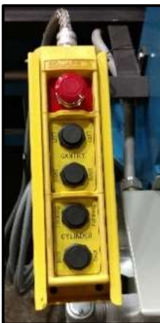
Operator's pushbutton control station is ergonomically designed, and features digital tonnage display and stroke control. Pendant-mounted controls allow positioning
