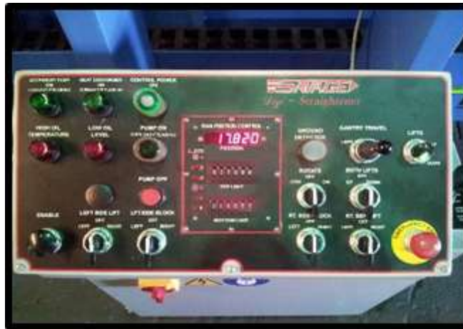
Operator's pushbutton control station is ergonomically designed, and features digital tonnage display and stroke control. Pendant-mounted controls allow positioning
