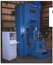
800 ton Slab Side Powder Compaction Press for GE Healthcare
