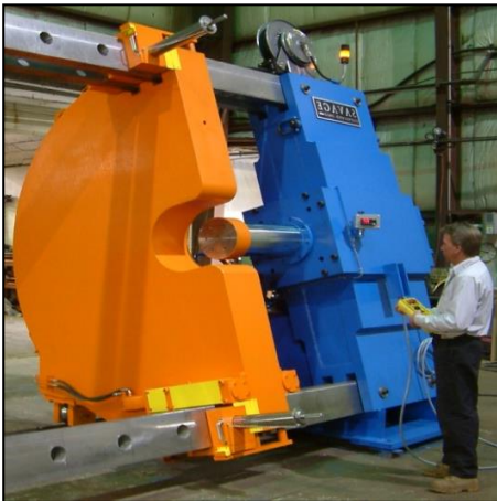
450 ton 90" Wide with Solid Plate Strongback for Tight Clearances between Gear and Housing
