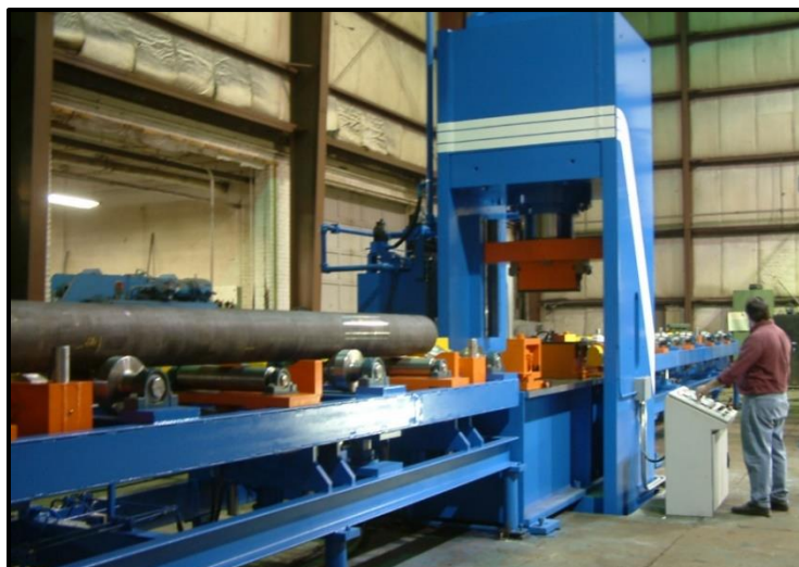
1800 ton Hybrid Press for Straightening Forged Stainless Steel Bars up to 18" Diameter
