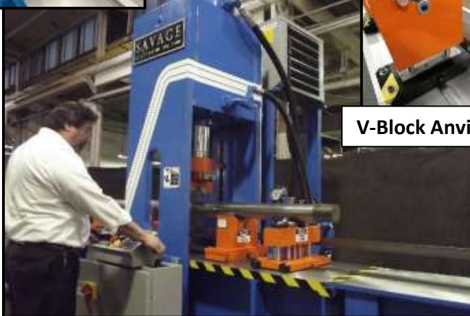
Ergonomic Operator Controls and Ram Positioning Controller for Precision Straightening
