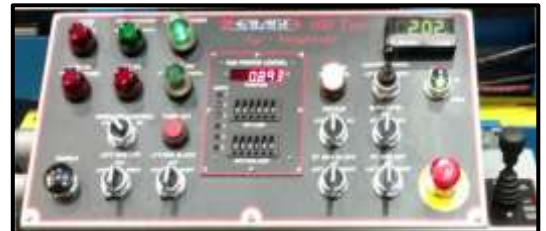
Ergonomic Operator Controls and Ram Positioning Controller for Precision Straightening
