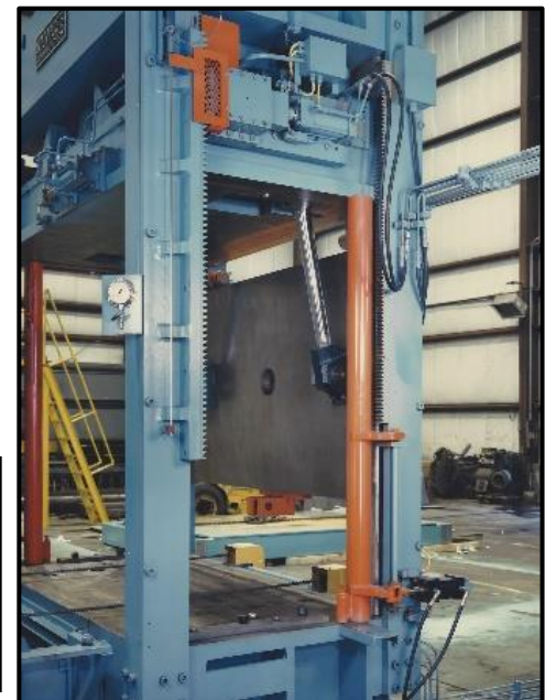
90° Rear Swing-Out Platen (96" x 68") with Frontal Shuttle Bolster
