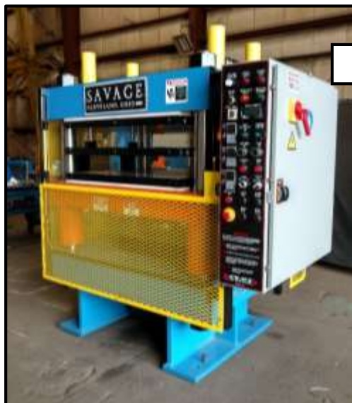
Line of presses for molding composite sabots for armor-piercing projectiles. Sabots are heated via infra-red source.
