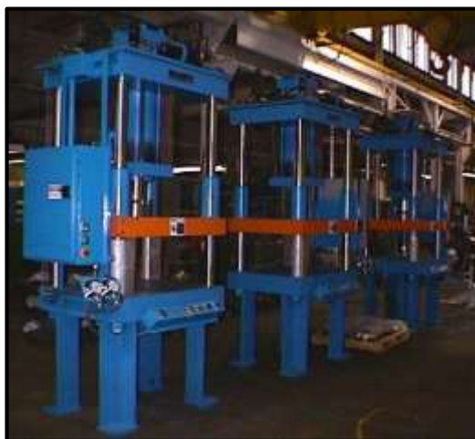
Line of presses for molding composite sabots for armor-piercing projectiles. Sabots are heated via infra-red source.
